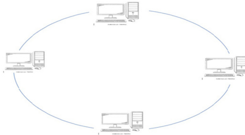
Figure 5: LAN with Ring Topology
